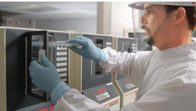
Technologist Jerry Davis uses a dynamic incubator for an EIA test at Knoxville in Tennessee, USA.
