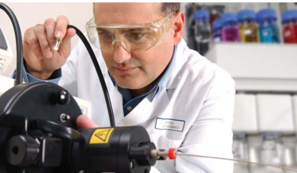
Scientist Peter Soupourmos with a mass spectrometer used to analyse proteins and peptides at Parkville in Melbourne.
