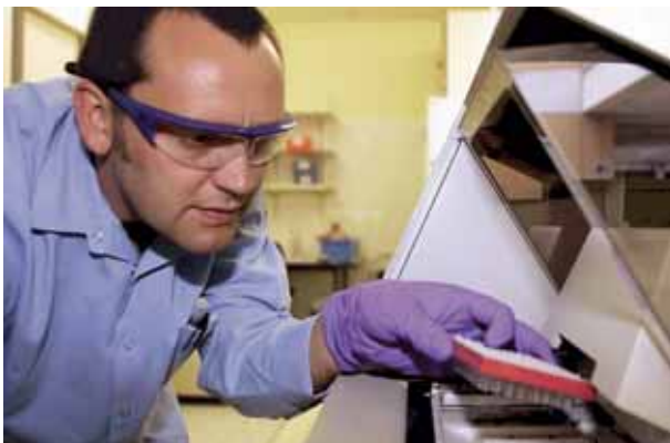
Laboratory technician, Thomas Rein, carries out a Real Time PCR quantitative virus detection assay used to determine that biological materials are virus free.
