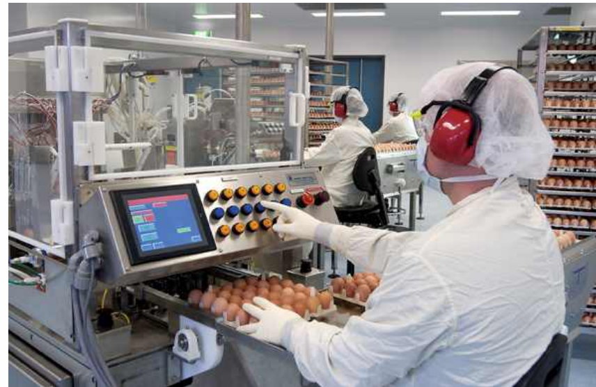
Egg harvesting machine in CSL's new state-of-the-art influenza vaccine centre
